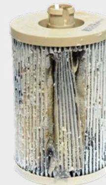
Figure 29 Use of elevated biodiesel blends requires consideration of potential operational implications
