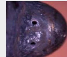
Non-Detergent Diesel This injector accumulated 8,800 MWhrs on non-detergent diesel only.
